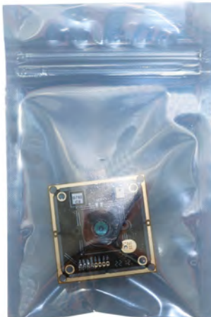
Place Camera Sample into Anti-Static Bag
